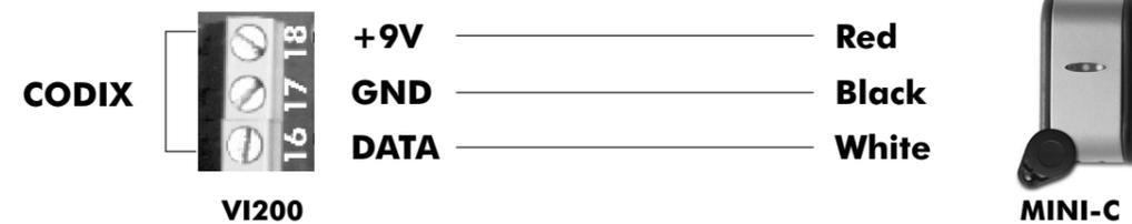
NOTE: Possible to connect a maximum of 3 readers (MINI-C) to one Control unit (VI200)
